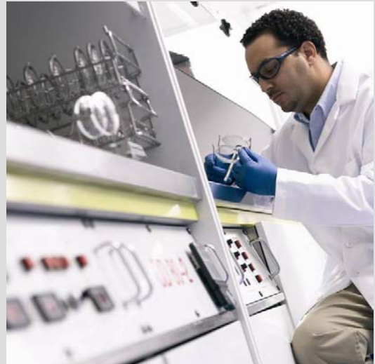
Applications Technician Terry Graham is preparing optical lenses to apply one of Nanofilm’s self-assembling nano-coatings, which is less than ten nanometers in thickness and provides a more durable protective coating to resist soiling and stains. Image courtesy of Nanofilm, Valley View, OH.
